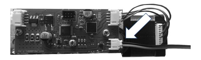
11. The slots on the motor assembly corresponds with the slots on the end of the exit device. Slide the motor assembly into the end of the device.
