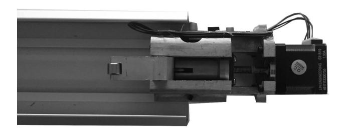
12. Slide the motor assembly into the bar, so it is within 1/8 of an inch from the end cap bracket when the push bar is depressed. Make sure that the push bar can move up and down freely with out anything coming in contact with the motor assembly.
